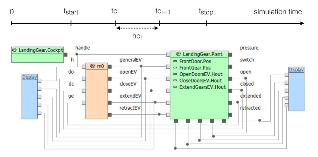
Simulation is broken down into communication steps  $tc_i \rightarrow tc_{i+1}$  of the size  $hc_i = tc_{i+1} - tc_i$
